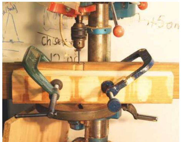
▲ Pic.14 Setup for drilling for the pin
